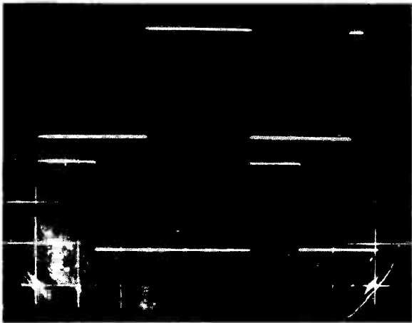
Fig. 7. Square wave output (above) with 2.5mS pulse output (below) at a repetition rate of 100Hz
