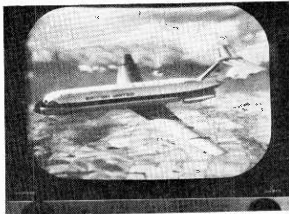
A monitor picture from a TV camera using a EEV sidicon tube to view a photograph under normal room lighting conditions
