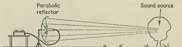
Fig. 2. A better method of obtaining birdsong recordings using a parabolic reflector. Note that the microphone is turned away from the sound source and towards the reflector dish
