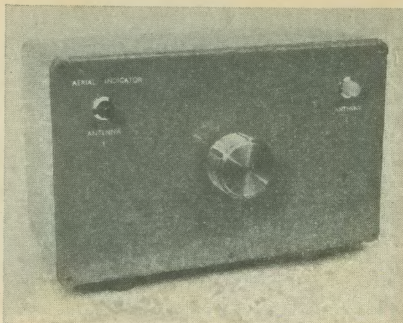
The front panel of the completed change-over unit PL1 is at the left and PL2 at the right
