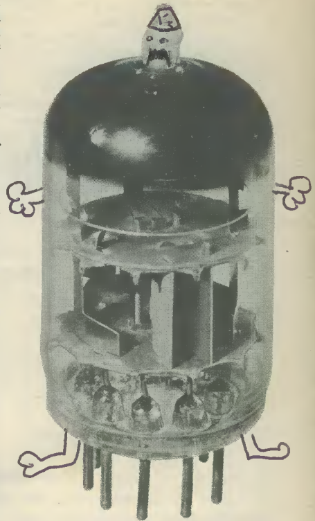
An example of present day construction. This valve, the PC88, operates as a grounded-grid triode amplifier at frequencies of the order of 850 Mc/s in u.h.f. tuner units for 625 line television receivers. It offers a fitting contrast to the ORA valve (circa 1920) which forms the heading illustration
