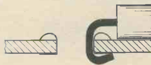
Fig. 3. Soldering a component lead-out to the tightened eyelet
