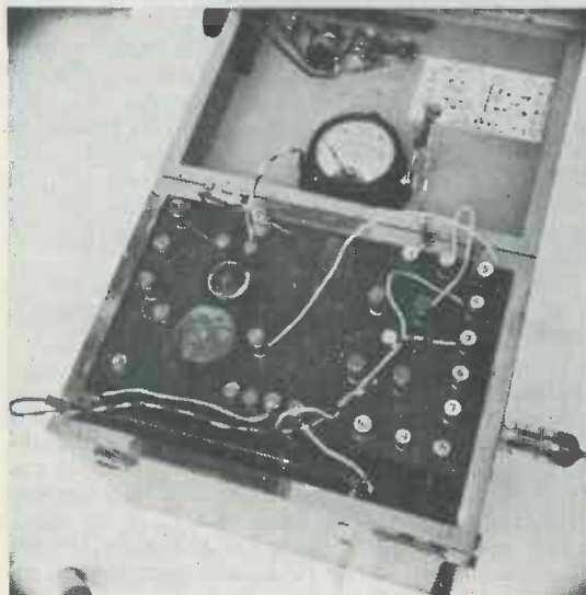
Testing the triode section of an ECL80
