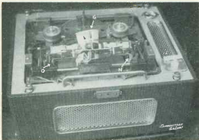
The deck with large mounting plate removed. Note the cigarette packet in G inserted between the plate and the capstan to prevent damage. The head leads can be seen at O and N
