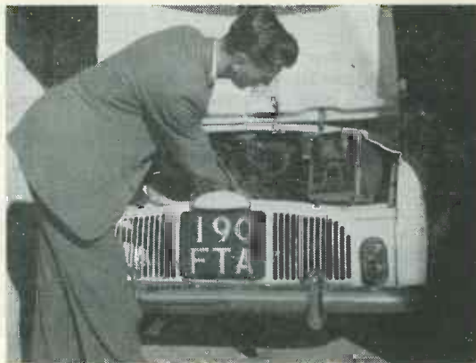
Testing an ignition system. The author's assistant examines the waveform at the distributor
