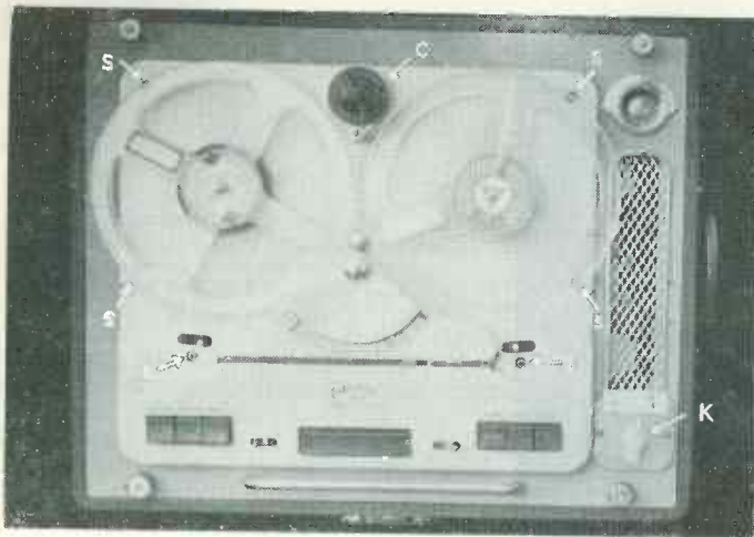
Top view of recorder. K is the new head switch knob. The plastic cover is removed after taking out the six screws at S and the speed control knob C.
