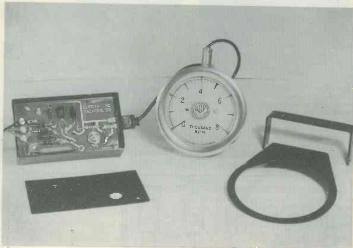
The complete unit wired and ready for testing
