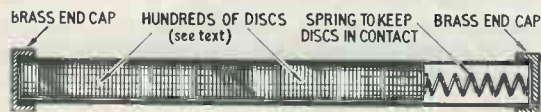
Fig. 2. Diagram of a Zamboni pile. About eight of these piles are used in a typical surplus image converter
