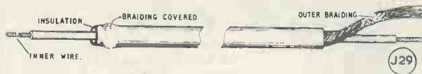
Fig. 29. Preparation of the ends of the screened wire. The first example shows the end of the braiding covered with the outer insulation, the earth connection not being required
