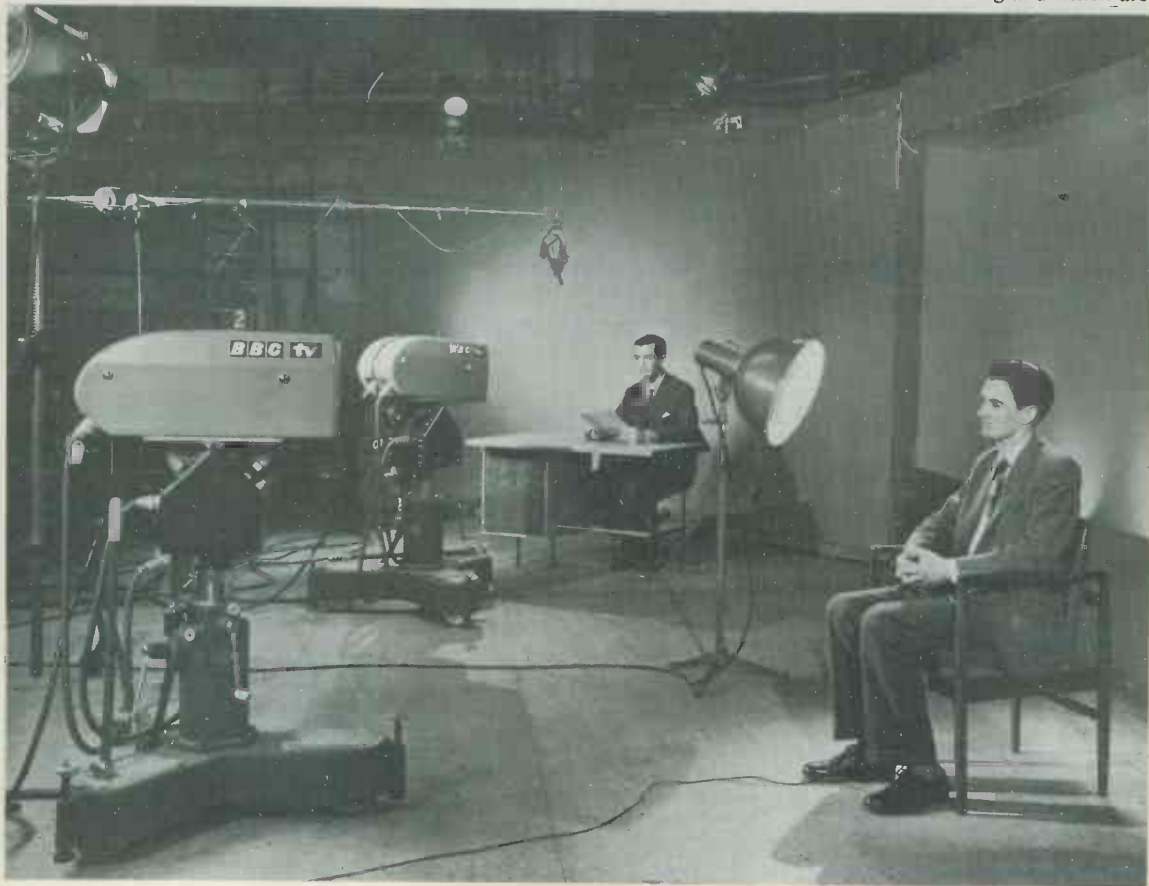
B.B.C. robot cameras in-action. These two cameras are remotely operated from the vision control room
