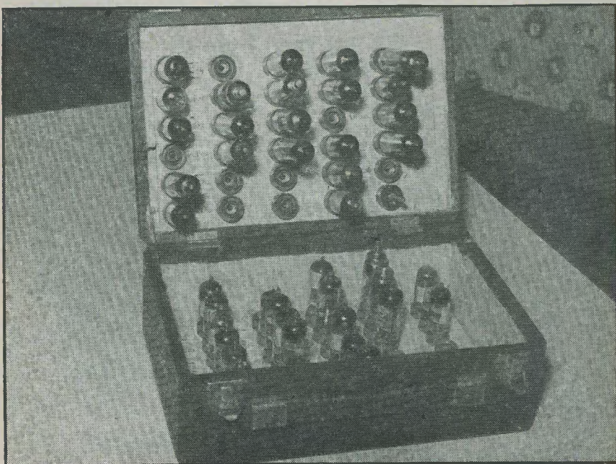
Photograph. A view showing the interior layout of the "Valve Caddy"
