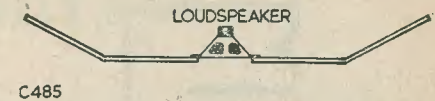
Fig. 6 If all four sides of a square baffle are folded back as shown, cabinet resonance should be almost entirely eliminated and the effective size of the baffle can be increased.
