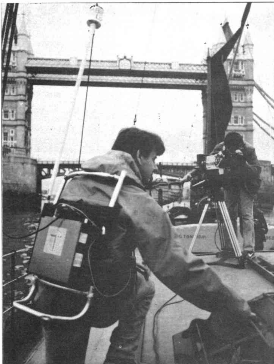
Microwave TV goes portable at Tower Bridge, London. A British Telecom engineer with backpack transmitter supports an electronic news gathering team from ABC-TV (USA)
