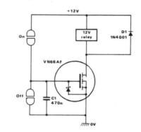
Fig 17 Semi-latching touch-activated relay switch
