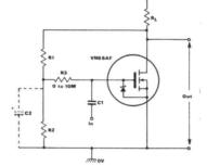
Fig 24 Biasing techniques for linear common source mode
