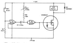
Fig 19 Simple relay output timer circuit
