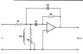
Fig 2 The tunable bandpass filter
