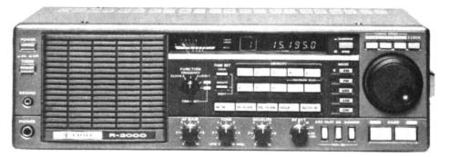
hour format, clock 1 being employed to operate a timer which will switch the receiver on/off at predetermined times, and clock 2 for local time or UTC as desired. With this facility it is possible to record an item which might be broadcast when one is otherwise engaged. The timer will switch on the receiver and also (by means of the 'remote' terminal at the rear of the receiver) switch on a cassette recorder. It will then switch both units off at the appropriate time.
