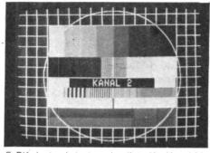
FuBK electronic test card radiated by Kanal 2 in Denmark
