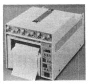
innovative writing system which has a special linear thermal array head, with inline heating elements placed at a rate of 6 dots/mm across the 4-inch chart width. A microprocessor-based drive system determines which elements will respond to the multiple inputs appropriate to each line.
