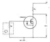
Fig 10 Basic VMOS digital switch or amp
