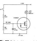
Fig 22 'Soft-start' lamp switch
