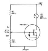
Fig 21 Simple dc lamp dimmer
