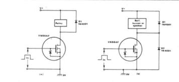
Fig 15 If inductive loads are used in digital switching circuits protection diodes must be connected
