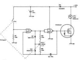
Fig 23 High-efficiency dc lamp dimmer
