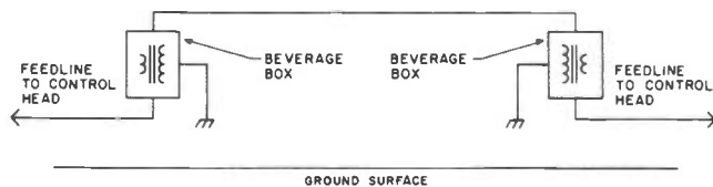
Fig 3 The directivity pattern of the K1VR/N1RC Beverage is reversible. A control head at the operating position selects one of the two feedlines and routes it to the receiver while terminating the second feedline with a resistance. The antenna is directional towards the end with the terminated feedline. By using three such antennas and a rotary switch six different directions can be selected
