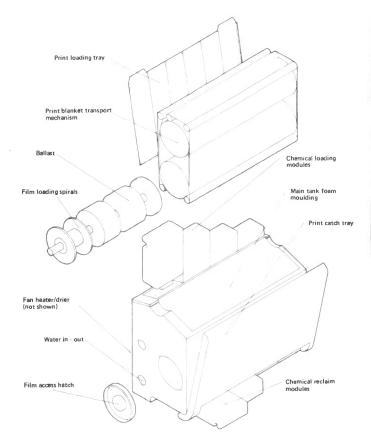
Figure 4: Component layout — exploded view.
