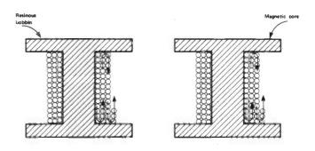
Figure 13: Multilayer solenoids. The arrows indicate the order of the turns.
