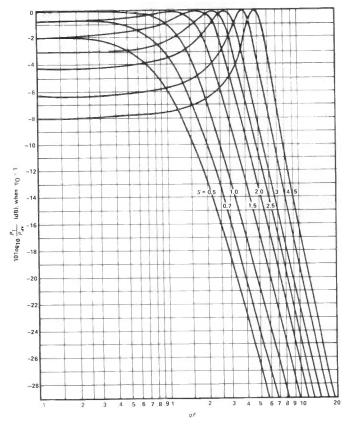
Figure 9: Relationship between qF and the power ratio.
