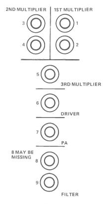
Figure 2: The transmitter tuning coils.
