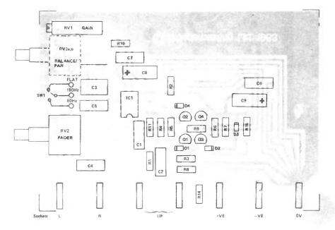
Figure 2: Component overlay for input amplifier.
