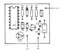
Figure 6: Component overlay for 4020based toneburst.
