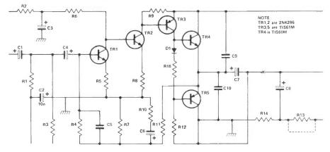
Figure 7: Circuit diagram for the audio amplifier.
