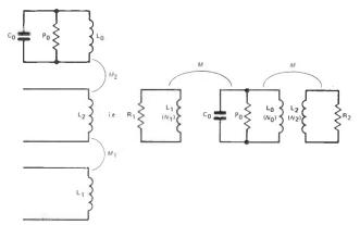
Figure 4: Equivalent circuit for a single-tuned band filter.
