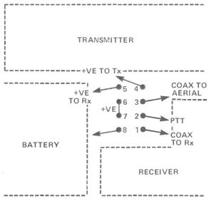
Figure 1: Connections from the relay (looking from PCB side).
