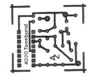
Figure 5: PCB for 4020-based toneburst.
