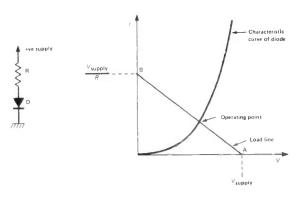
Figure 5: Determining the operating point of a resistor/diode circuit.
