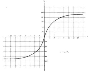
Figure 7: Phase angle-frequency characteristic for a singletuned band filter.
