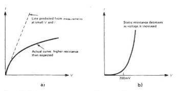
Figure 2: Voltage/current graphs of two non-linear devices. a) Filament bulb; b) Silicon diode.
