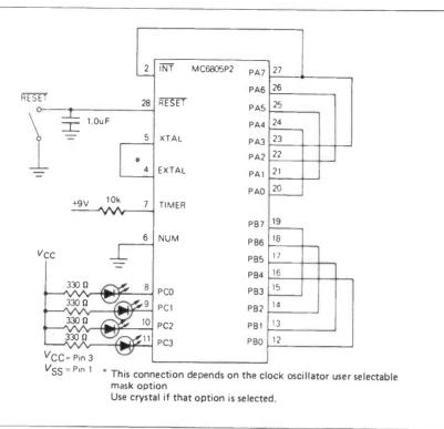
Figure 3: Self-check connections.
