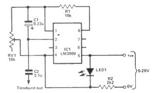
Figure 1: Manually timed toneburst circuit.
