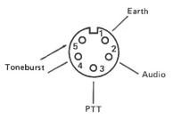
Figure 6: Pin connections for the mic/ speaker plug.
