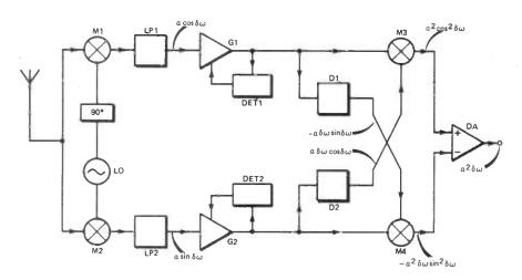
Figure 2: STC's suggested approach to coil-less FM radio.
