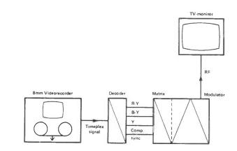
Figure 6: Line picture play back with RF-modulator.
