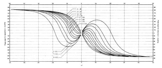
Figure 11: Relationship between qF and phase angle.
