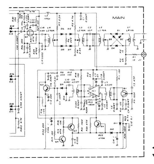
designer has discovered (like we all do) that an undecoupled noise blanker can actually introduce more noise than it removes. The emitter of Q3 is also heavily decoupled via C12, since this comparatively long lead would provide an excellent additional noise source if given the chance.
