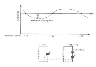
Figure 1: The classic '3 point tracking' compromise for making the best of the inevitable difference between the resonant frequencies of an antenna and an oscillator coil.
