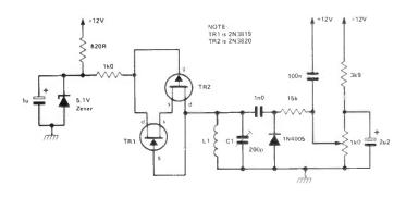
Figure 11: Varactor controlled oscillator incorporating a Lambda diode.
