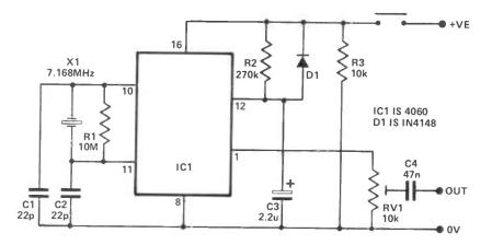
Figure 3: Circuit for the toneburst generator.
