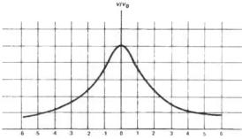
Figure 6: Amplitude-frequency characteristic for a single-tuned band filter.
