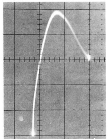
Photo 1: Oscillograph of Lambda Diode characteristic curve as obtained from a curve tracer. 1mA/division in y; 2V/division in x
