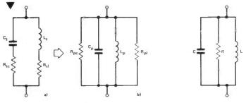
Figure 2: Equivalent circuit based on the coil constants.
