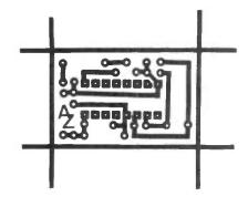
Figure 5: The toneburst PCB foil pattern.
