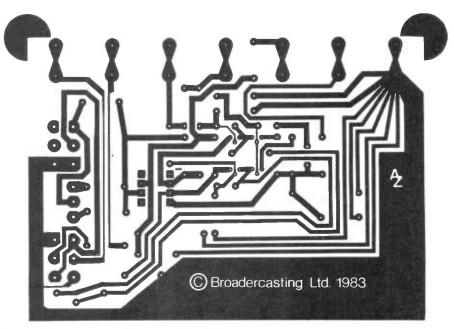
Figure 1: Foil pattern for input amplifier PCB.
