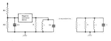
Figure 7: Simple negative resistance oscillator and equivalent AC circuit.
