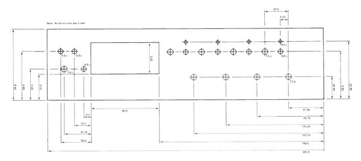
Figure 6: Front panel piercing instructions. Note that the phono jack socket has been moved to the side panel.
