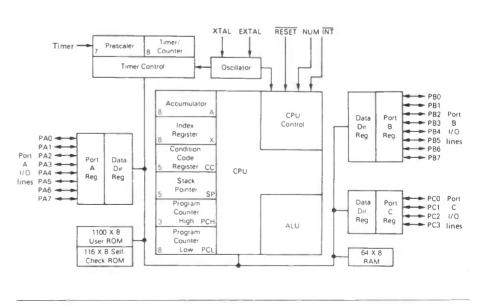
Figure 2: MC6805P2 HMOS microcomputer block diagram.
