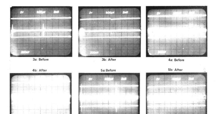
Top = noise blanker gating signal Middle = actual noise pulse after IF filter Lower = actual noise impulse fed to the receiver input
