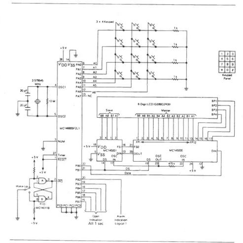
Figure 4: Digital lock system schematic diagram.
