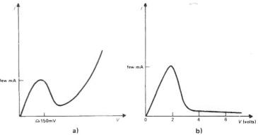
Figure 3: Voltage/current graphs of two negative resistance devices. a) Tunnel diode; b) Lamdba diode.
