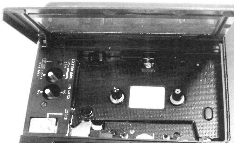
Inside the cassette compartment, showing Dolby, EQ and bias switching.
