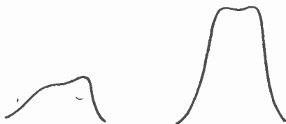
FIGS. 135 and 136.—On the left is seen the effect of heavy damping on an I.F. circuit, and on the right how it appears when the damping is removed.
