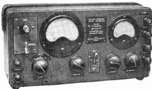
Fig. 5.—This is a Valve Voltmeter for battery operation. The General Electric Company supply this model.
