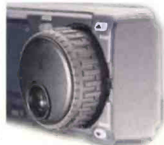
Fig. 3: The main tuning knob has a friction brake which increases the tension on the knob which Richard GORSN says makes a big difference when you are operating from the car.
