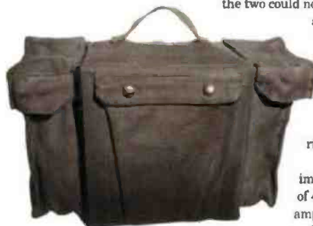
Fig. 4: The No. 128 carry case, pockets at each end hold headphones, microphone and leads. Crystal are held in little pockets behind front flap.
