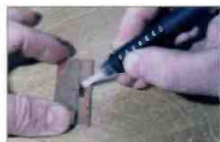
Fig. 1: The Resistance Unit (RU) 'pen' in action. The fluid flows through minute holes from the 'nib' onto the copper (see text).
