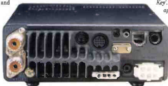
Fig. 4: Rear panel of the MkIIIG showing the two antenna connections, microphone and key connections and 'EXT' speaker connector.
