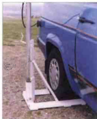
Fig. 5: The prototype 'TEX' version in use with the Reliant three wheel car. The mast is about to be 'locked' into the vertical position with the top clamp (note that prototype was painted, the production version will be 'hot dipped' galvanised (see text)).
