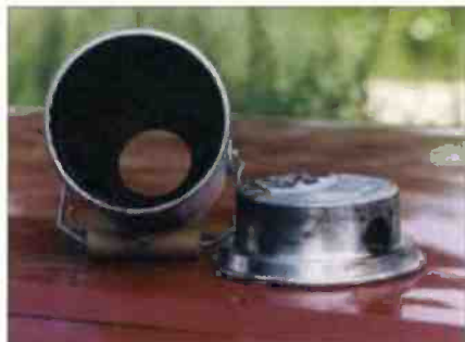
Fig. 9: The 'secret' of the 'Kelly's Kettle' is the remarkably large heating surface area. It will boil your water very quickly and you can soon be back on the air!
