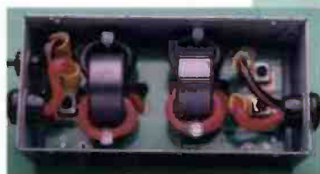
Fig. 7: The EMC filter box of the Icom IC-706 MkIIIG and (inset) the inside view.
