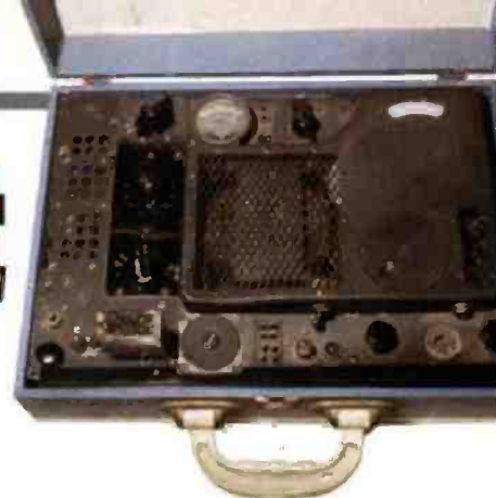
Fig. 1: The No. 121 Set. Receive tuning dial top left, transmitter on right, Morse key lower right.
