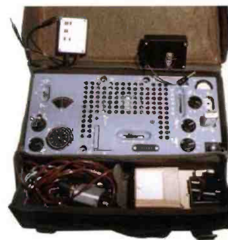
Fig. 2: The No. 123 Set. Receive on left, p.s.u. in centre, transmitter on right, Morse key lower right of set.
