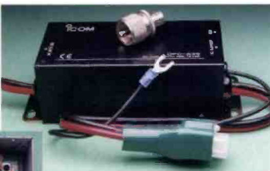
Fig. 7: The EMC filter box of the Icom IC-706 MkIIIG and (inset) the inside view.
