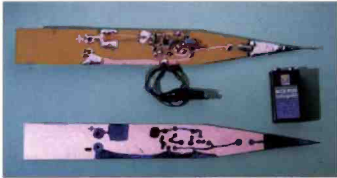
Fig. 2: Photograph of a completed 'Basi-Probe' (top) complete with probe tip (see text) and grounding lead complete with crocodile clip. The capacitor shown at the 'probe' end is C3, the coupling capacitor used to apply the test signal to the unit on test. The narrow (spear shaped) section of SRPB material forms the on-off switch (see text). The lower part of the photograph shows a 'Basi-Probe' before etching. The large etch resist covered area at the probe end will provide a secure mounting area for the probe itself (see text).
