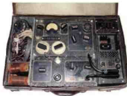
Fig. 6: The B2 spy set, the transceiver is top centre, the receiver is below, the p.s.u. is on the right side, spares box on left. (Photograph B. Warner).
