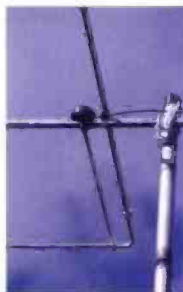
Fig. 2: A Gamma-match bar allows a good match to be made over part of the 50MHz band.
