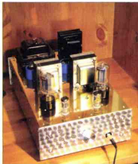
Fig. 4: A low power headphone (yes headphone!) amplifier. See text for further details.
