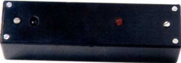
Photo 2: The remote receiver. The inset diode is the infra-red detector and the 'proud' diode on the right is the operating indicator (see text).
