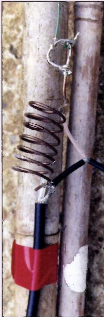
Fig. 4: Checking to see 'if it works' before committing yourself to buying an expensive fishing pole. (I've used the coaxial capacitor in this version).
