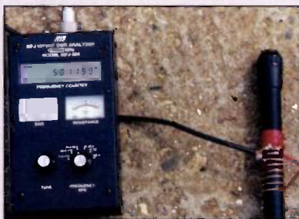
Fig. 2: The coil and fixed capacitor resonate at about 50.125MHz. The capacitor has its 'legs' insulated.
