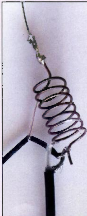
Fig. 5: A 'nude' version of the coil/capacitor for more detail.
