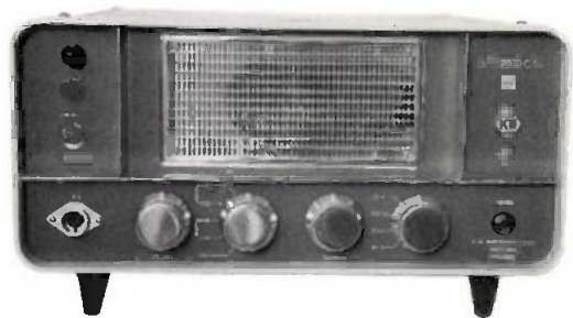
Fig.2: Ben G4BXD recently discovered this unusual transceiver, the KW2000CA, a 'special' four-channel crystal-controlled version of the well known Amateur Radio KW2000 transceiver (see text).
