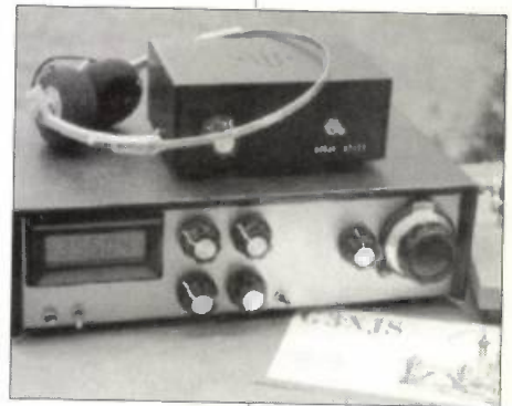
Home-brew QRP equipment can give great satisfaction when c.w. operating. This 3.5MHz transceiver has an additional digital frequency read-out and audio filter - the keyer on top is home-brew too!
