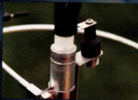
A close-up shot of the method of mounting the ringbase elements, and the coaxial feedpoint devised by Sandpiper Communications.
