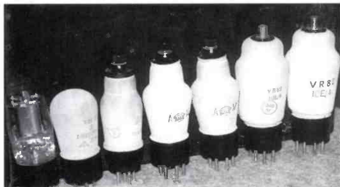
Fig. 5: Some of the valve types used in the RAF R1116 receiver. The receiver used 2V and possibly 150V h.t. supplies (see text).
