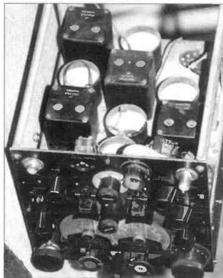
Fig. 2 (Right): The hooded illumination provided for the tuning dials on the R1116 is a distinctive feature on this design (see text).
