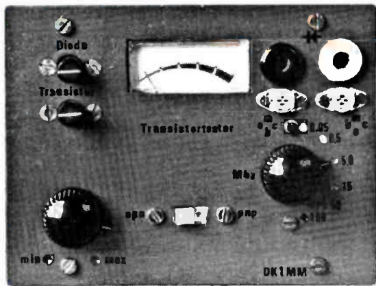
Fig. 1: The prototype bi-polar transistor tester as built by Martin Michaelis DK1MM.
