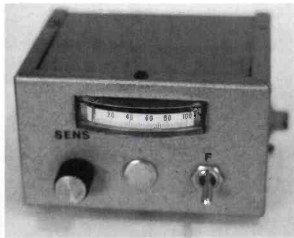
Fig. 2: The completed and assembled enclosure, made with the 'U' method.
