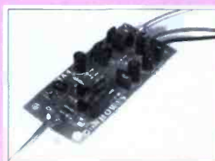
The completed Howes MA4 microphone amplifier kit.
