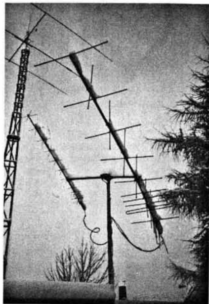
A "Christmas card" scene of the G3IOR satellite antenna system for 144 and 430MHz, well detuned by snow
