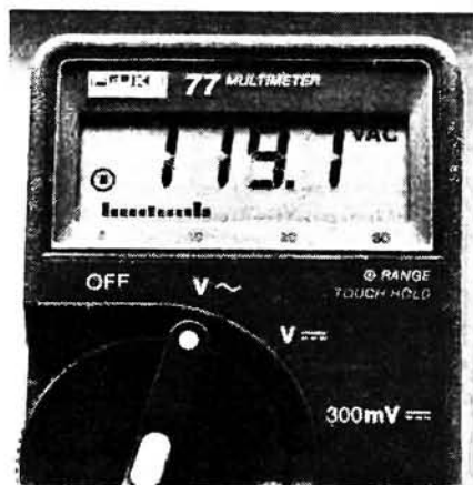
The Fluke 77 is an autoranging d.m.m. which incorporates touch-hold and automatic power-down facilities, and combines digital and analogue readouts for maximum versatility
