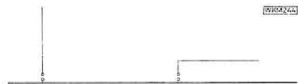
Fig. 2: The EMGA antenna is just the conventional quarter-wave vertical antenna formed into an inverted-L, the ratio of length to height determining the effective height
