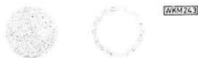
Fig. 1: Looking at the cross section of a conductor carrying direct current, left, the theoretical electron flow is even across the wire but with high frequency currents the flow is confined to the outer part, left
