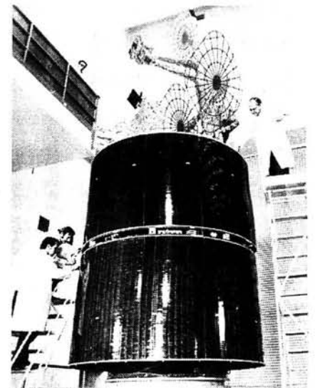
Fig. 1.3: An INTELSAT IVA cylindrical spacecraft being prepared for launch INTELSAT
