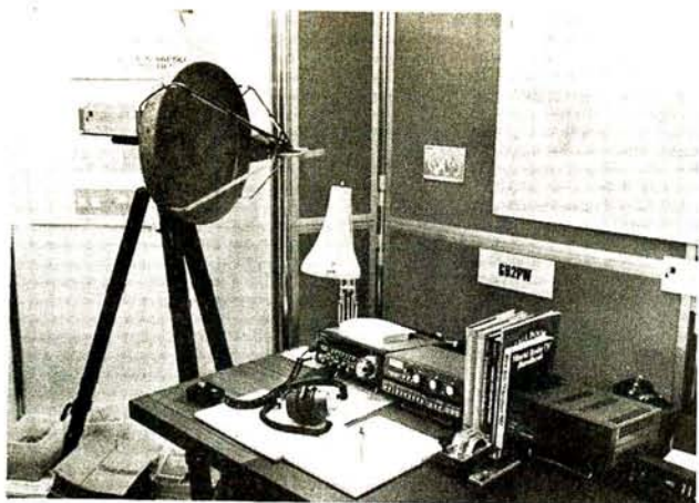
The h.f. station GB2PW, with our prototype microwave transceiver alongside it. The dustbin-lid antenna of the latter attracted a lot of attention from visitors to the exhibition
