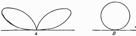
Fig. 8.—With the usual heights obtainable on Topband, the vertical aerial will radiate mainly horizontally, while the horizontal aerials will radiate mainly upwards.
