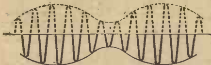
Fig. 2.—The result of half-wave rectification, the negative half-cycles have been suppressed.
