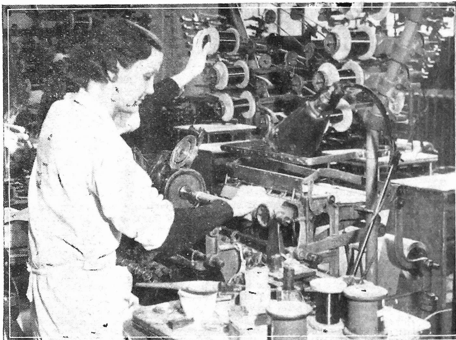
A woman operator at a complicated coil-winding machine in a British radio factory which is working at full pressure producing radio sets for the export trade.
