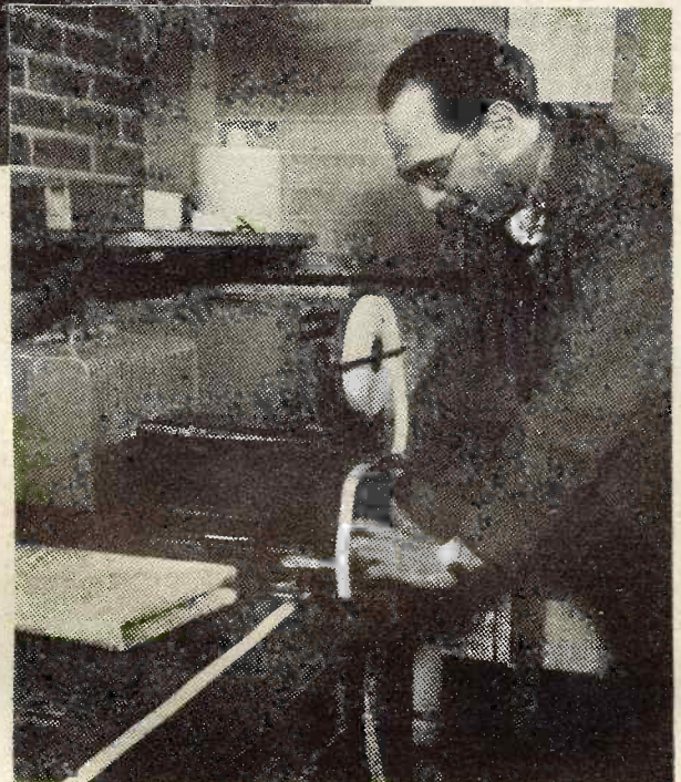
Fig. 2.—The Hellschreiber machine, that tapped Goebbels news and service instructions to his network of newspapers and broadcasting units.
