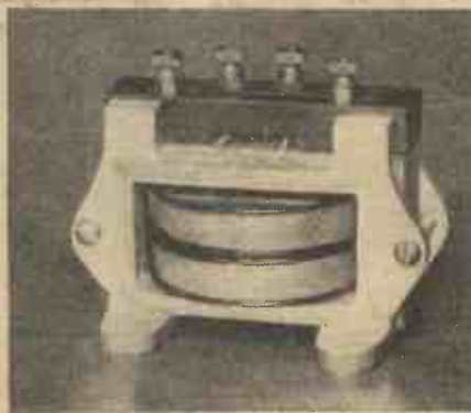
A small home-made transformer intended for use in a trickle charger. An output of only about 9 volts, 1 amp. (9 watts) is required, and therefore the transformer can be quite small.
