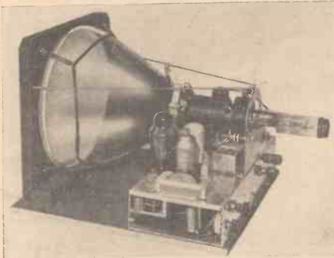
Fig. 1.—A 12in. Baird cathode-ray tube mounted with time-base generator chassis prior to incorporation in a complete receiver.
