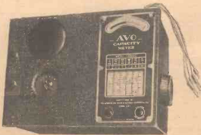
This illustration shows the new Avo Capacity Meter, and the six-section calibrated dial may clearly be seen. This particular instrument is designed for battery operation.
