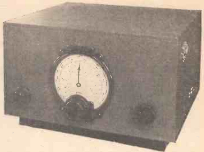
The Multiwave Three in a Laurence cabinet showing the single all-wave tuning dial.
