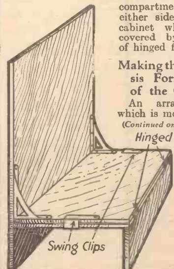
Fig. 4.—A chassis made in two pieces hinged at the back.
