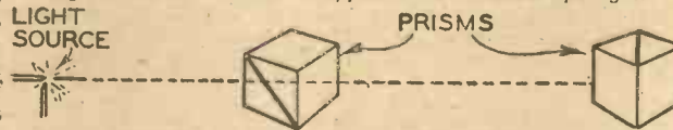
Fig. 3.—When the prisms are set up in this manner, no light passes.
