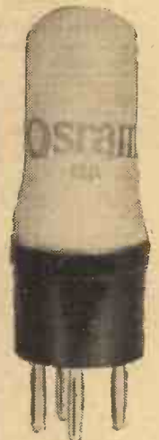
The new Osram "K" type valves referred to last week. The valve base is of standard size, and the smallness of the bulb may therefore be judged. The prices for these valves are the same as for the standard types.
