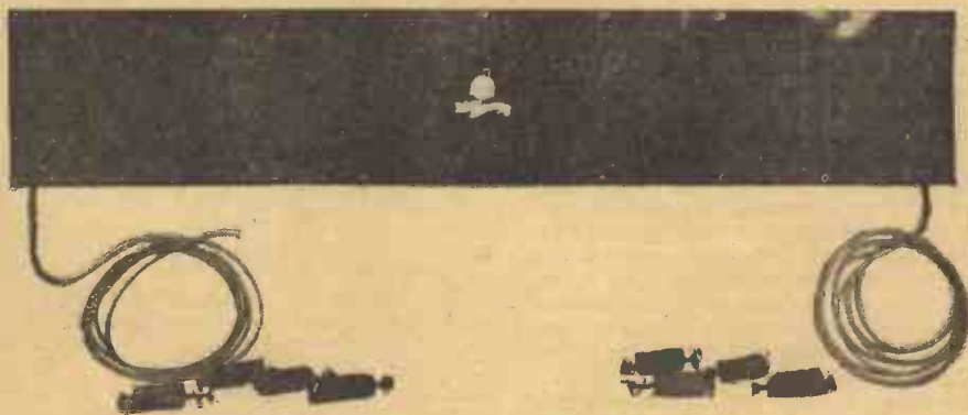
This aerial fitment is intended to be mounted below the running board.
