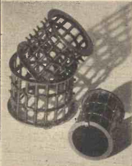
Here are the three special insulating forms with their moulded-in pegs for external connection anchorage. Note the air-spacing for windings, and the absence of paper, cotton, or other hygroscopic material which causes breakdown.
