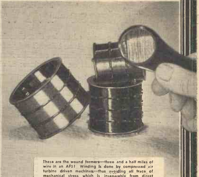
Here are the three special insulating forms with their moulded-in pegs for external connection anchorage. Note the air-spacing for windings, and the absence of paper, cotton, or other hygroscopic material which causes breakdown.
