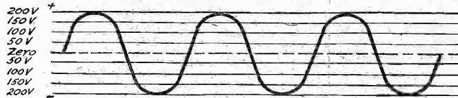
Fig. 1.—A graphical representation of the output from an A.C. supply; the voltage and polarity are constantly changing.
