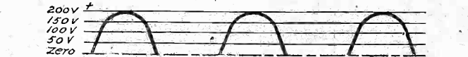
Fig. 2.—This graph shows the result of half-wave rectification; one half of each wave is eliminated.
