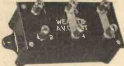
Fig. 1.—Photograph of A.V.C. unit.
