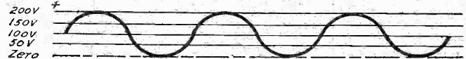
Fig. 3.—This shows the result of full-wave rectification. Both halves of the wave are made use of to produce a voltage of uniform polarity.
