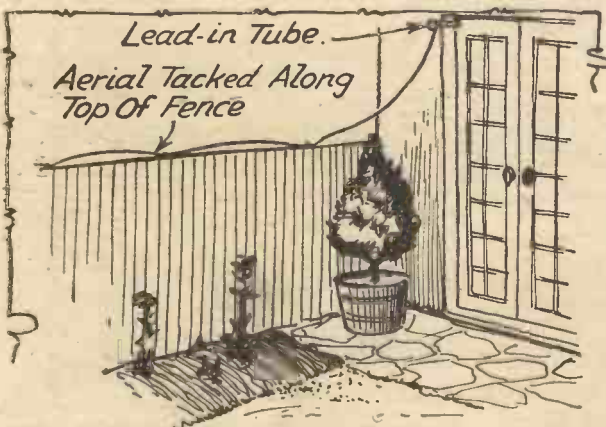
Fig. 2.—When the aerial collapses, the wire may be temporarily fixed along the top of a wooden fence.
