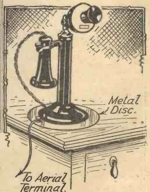
Fig. 5.—A temporary aerial system formed by capacity coupling with the house telephone system.
