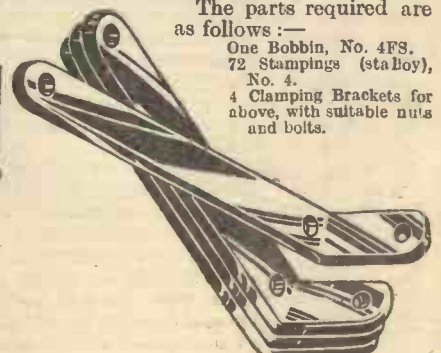
Fig. 5.—The stampings and clamping brackets.
