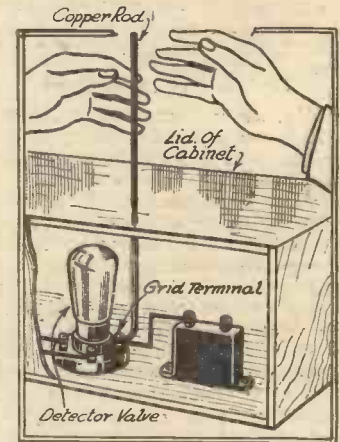
Fig. 1.—How the "radio violin" is made and played.
