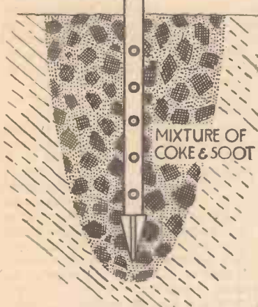
Fig. 1.—A cheap, simple, but very efficient earth.
