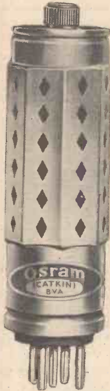
The new Catkin valve. Note the metal envelope, which forms an air-cooled anode. This illustration shows type V.M.S.4.
