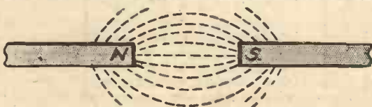
Fig. 2.—The lines of force set up between two magnets.
