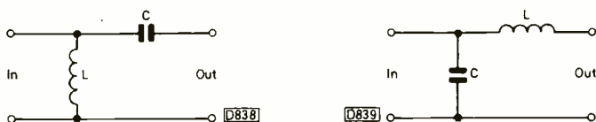
Fig. 1 (left): Basic high-pass filter.
