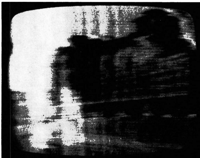
China ch. R1 received in Holland by Ryn Muntjewerff via F2 propagation. Note the smeary video image.
