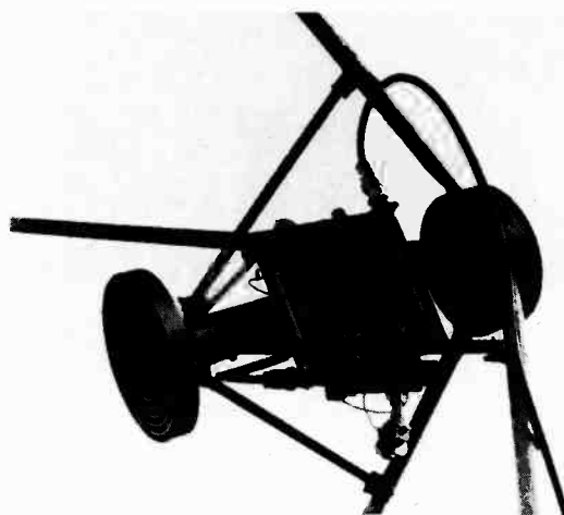
Close-up view of S. Birkill's 11.6GHz head unit, mounted at the focus of an 8ft. dish.
