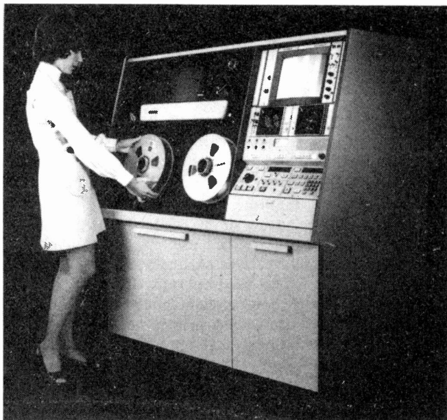
The Ampex Model AVR-3 is the world's first "intelligent" VTR. The AVR-3 allows broadcasters to record and play back live pictures automatically. When equipped with the optional edit controller the AVR-3 can be programmed to handle a wide range of editing functions otherwise currently possible only with computer editing systems. The AVR-3 is a dual-band machine compatible with existing broadcast equipment.
