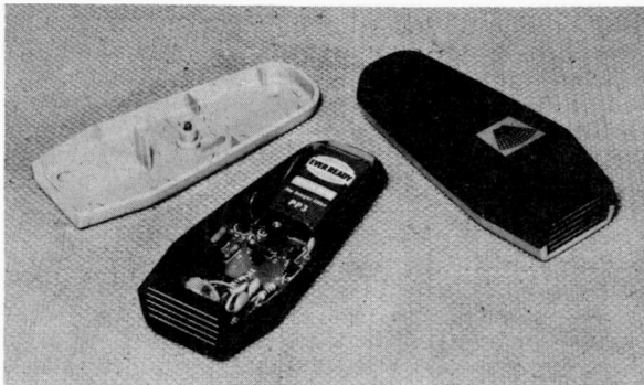
Photograph showing details of the hand-held ultrasonic remote control transmitter unit.
