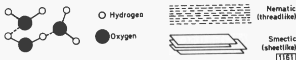
Fig. 3 (left): Short range order in water. Each hydrogen atom attracts the oxygen of another group enough to cause some order so that water boils at a fairly high temperature.
