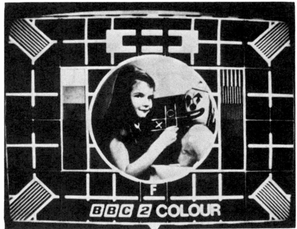
Off-air test card photograph, showing the excellent linearity and good grey scale.
